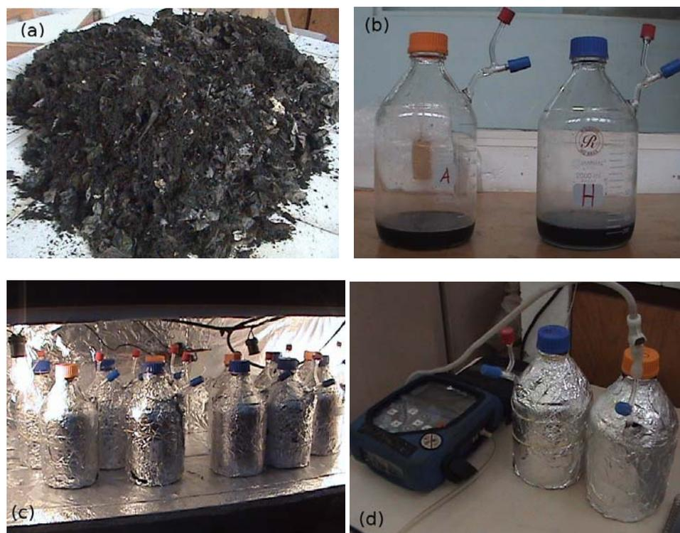
**Figure 8:** Materials used in the BMP tests. a) shredded waste; b) bio-digestors; c) bioreactors in the chamber and d) biogas composition determination
