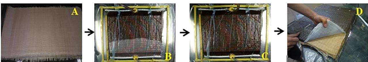
Fig 1. a) Fabric stacking; b) Initial resin flow; c) End of reinforcement filling; d) Composite demolding.
