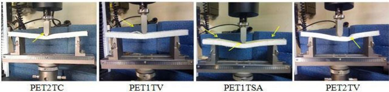
Fig. 6. Samples behavior after flexural testing.
