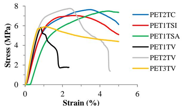
Fig. 5. Stress versus Strain curves in flexural testing.
