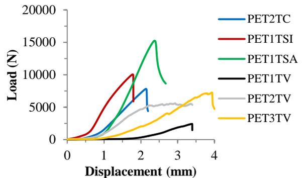
Fig. 3. Load *versus* Displacement curves of different sandwiches for longitudinal compression testing.
