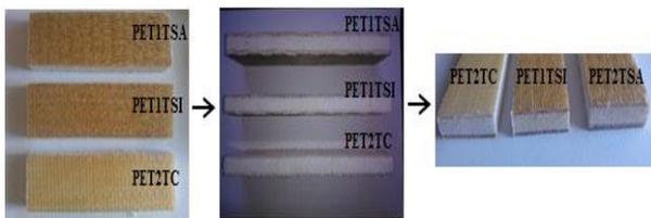
Fig. 2. Sandwiches composites reinforced with sisal fabric (PET1TSA, PET1TSI e PET2TC).
