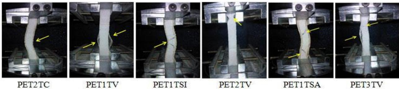
Fig. 4. Behavior of the samples during longitudinal compression testing.
