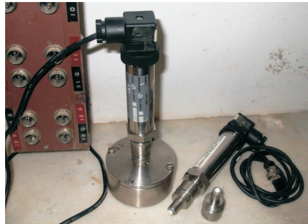
Figure 1 - Vaporization chamber used in the first set of tests, tensiometer and porous tip.
