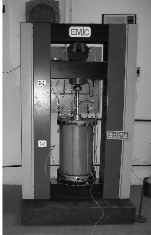
Figure 3. A view of employed loading frame and triaxial chamber
