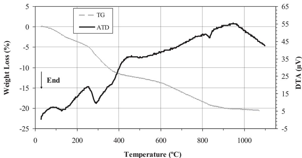
**Figure 1. TG/DTA curves of the red mud as received**
