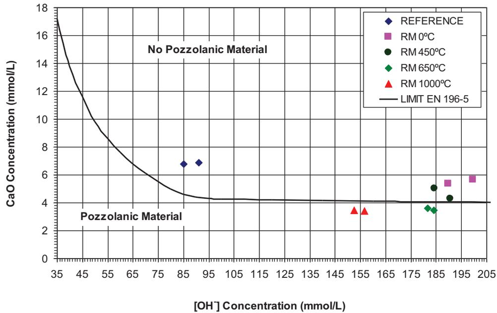
**Figure 4. Diagram for determining the pozzolanicity according to NP EN 196-5 standard**
