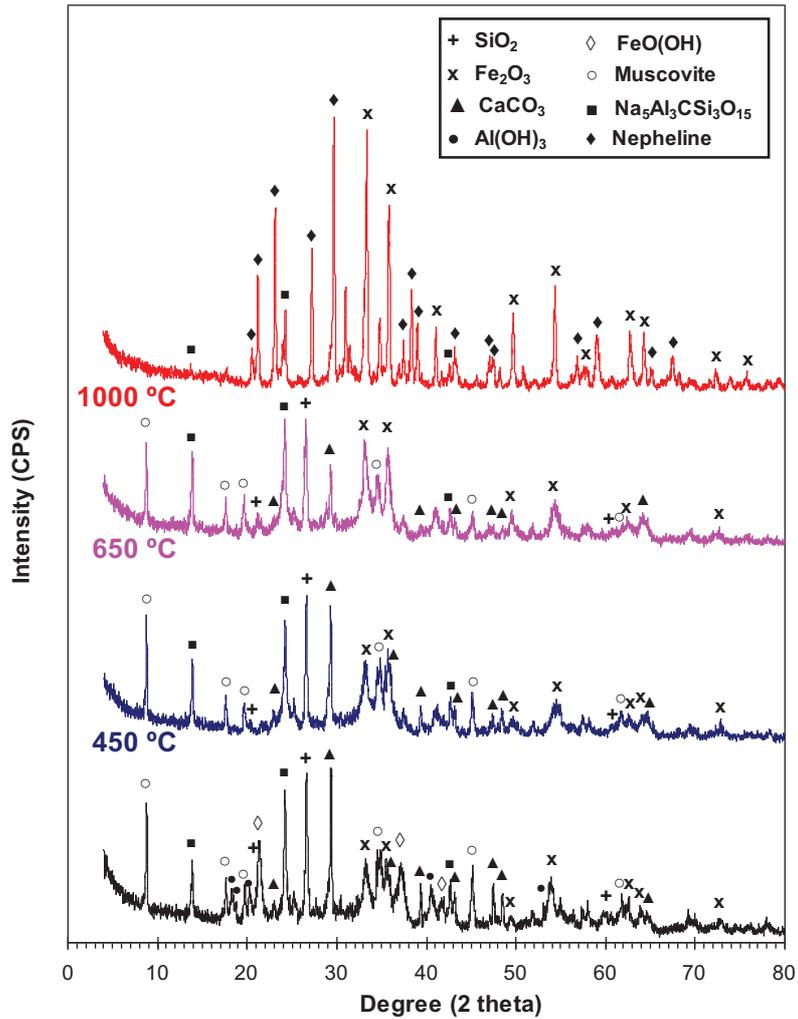
**Figure 2. X-ray diffraction patterns of the red mud as received (lowest curve) and after calcination at 450, 650 and 1000°C**
