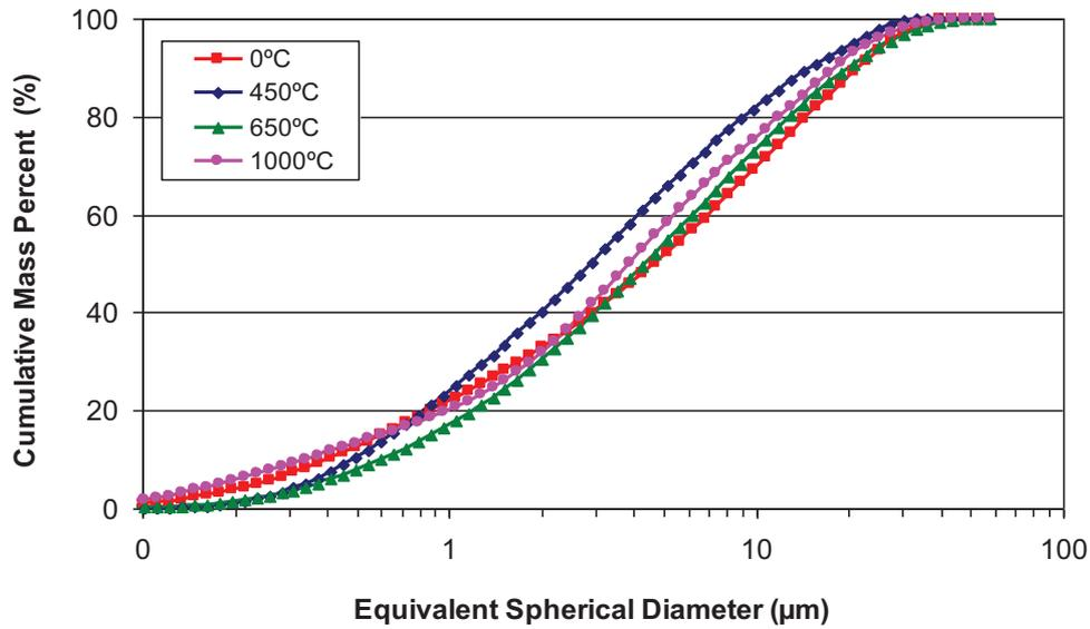
**Figure 3. Particle size distribution of the red mud as received and after calcination at 450, 650 and 1000°C**
